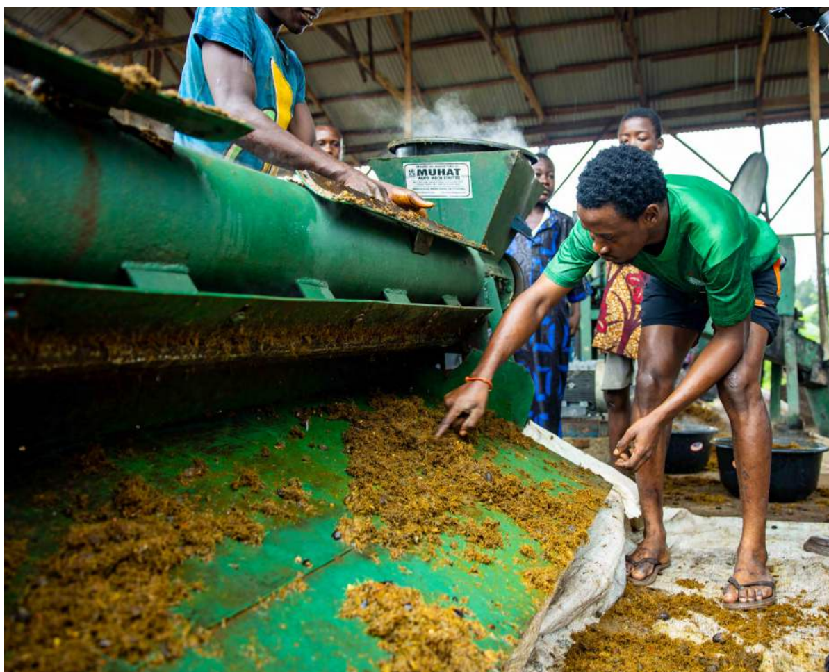
Technician at the Adebayo mini-factory operates the nut-fiber separator. Photo credit: TNF Media
